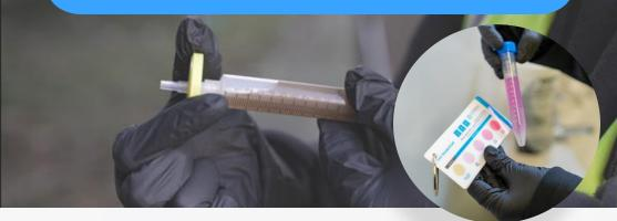
Our products show an immediate visual color change when in contact with Uranium, Plutonium, Americium, Cobalt and Primary Transition Metals at trace levels.
